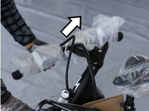
Ensure that they are fully extended and that the handlebar release latch is fully locked into place.
