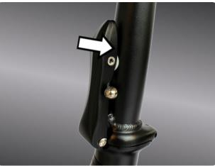
Carefully unfold the bicycle, from the center hinge, into the fully straight position. Make sure the frame release latch is firmly pressed towards the frame until it is securely locked into place.
