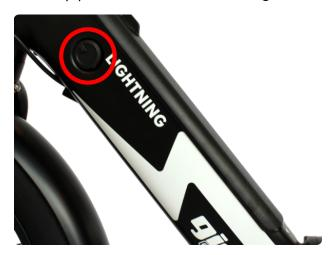
Locate the charging port cover on the side of the frame and flip the cap open to reveal the charging port or if charging off the bike locate the port directly on the side of the battery. ALWAYS plug your charger into the battery FIRST and THEN to the wall outlet. DO NOT plug a power cord already plugged into a wall outlet directly into the battery. The battery charger included is designed specifically for your Lightning e-bike, connecting the battery to any other charger will void the warranty.
